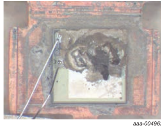
Fig 76. Sample image 4: source wires fused
