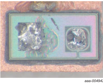
Fig 59. Sample image 68; 20 V, 3 A, 60 ms
