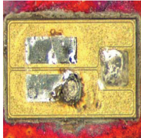
Fig 66. Sample image 2; 15 V, 2.5 A, 100 ms
