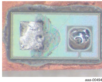
Fig 60. Sample image 69; 20 V, 3 A, 60 ms
