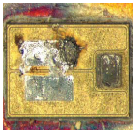
Fig 70. Sample image 12; 15 V, 5 A, 1 ms
